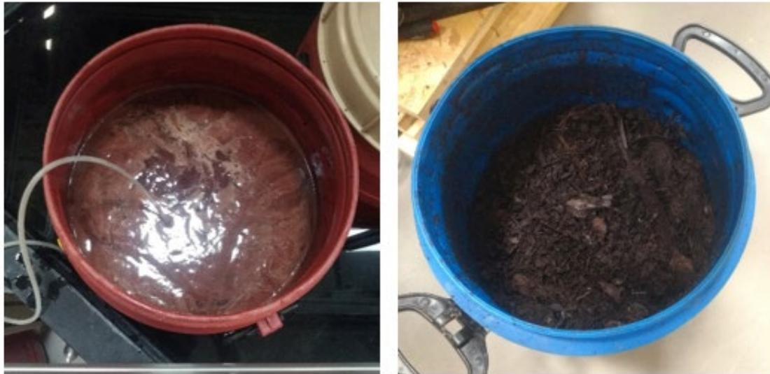
*Figure 9: Ammonium-Reactor and Compost. Ammonium-Reactor after addition of blood meal on day of experiment zero (left). Compost used as microorganism source (right).*
