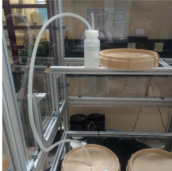
Figure 10: Gas-wash bottle installed to create anaerobic conditions.
