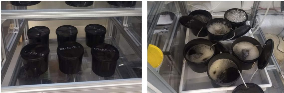
A-Figure 2: Left: Anaerobic Reactors. Right: Aerobic Reactors
